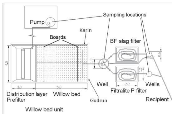
Fig. 1. Layout of the experimental wastewater treatment plant. Units are given in m.
