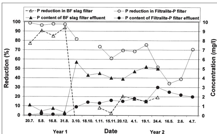
Fig. 7. The reduction and the effluent concentrations of tot-P in the adsorbents. The open marker denotes the reduction rate and the closed marker the effluent concentration.
