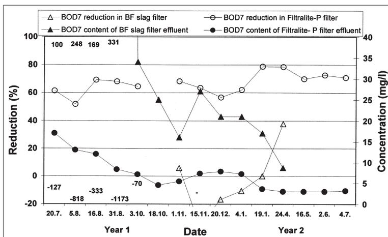
Fig. 8. The reduction and the effluent concentrations of BOD<sub>7</sub> of the P filters during the experiment.
