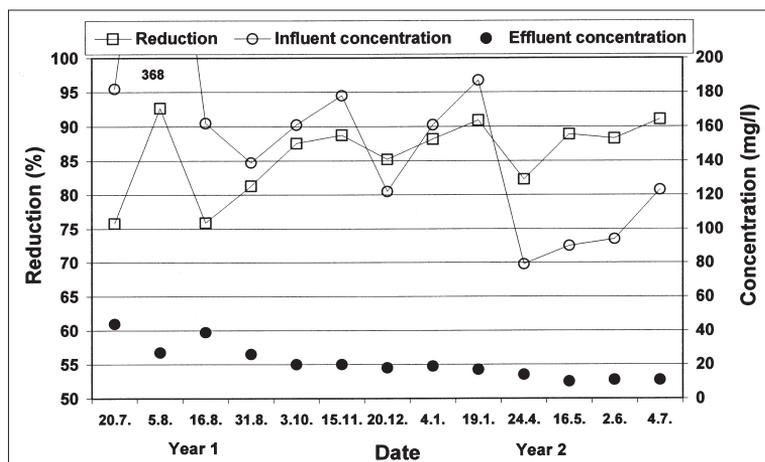
Fig. 6. The reduction and the effluent concentrations of BOD<sub>7</sub> in the willow bed during the experiment.
