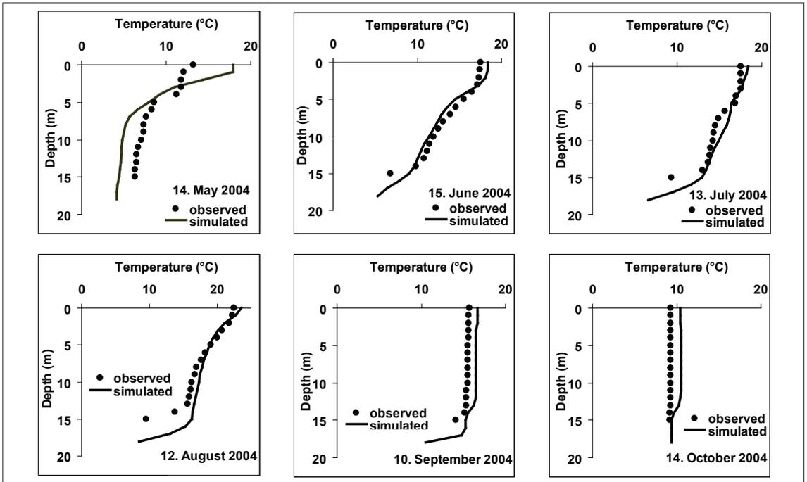
Figure 3. Simulated temperature in the water-column profile of the Aurevatn reservoir showed good accordance with real conditions.
