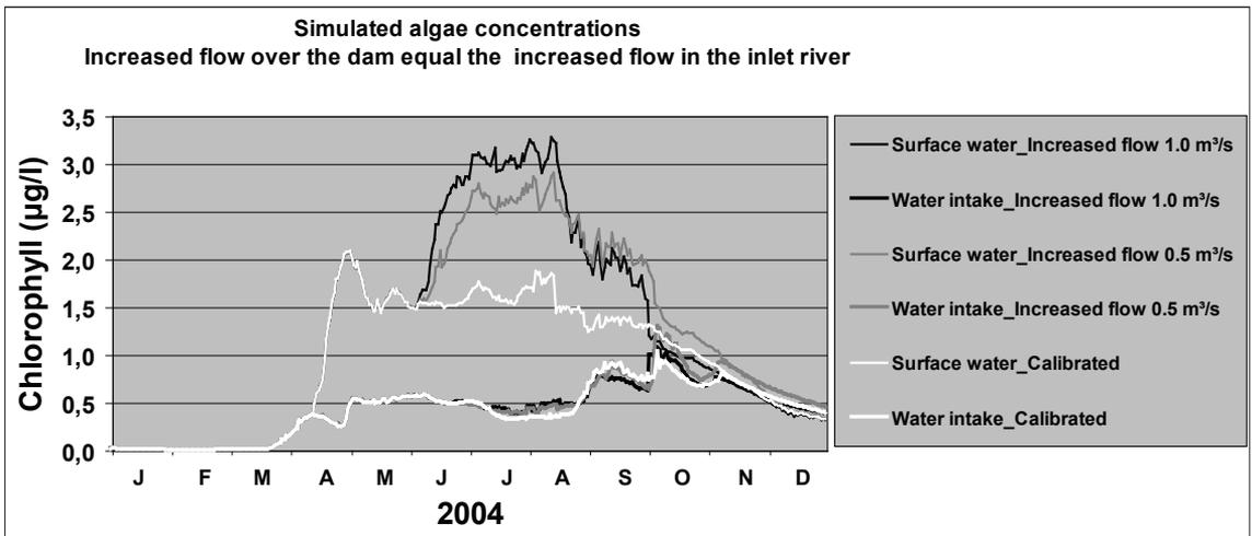
Figure 5. An increased discharge emptied over the dam equivalent to the volume of water in the upper-most meter of the Aurevatn reservoir involved a stimulation of growth of microalgae. An improvement for the quality of the raw water would not be obtained by this hydraulic operation.
