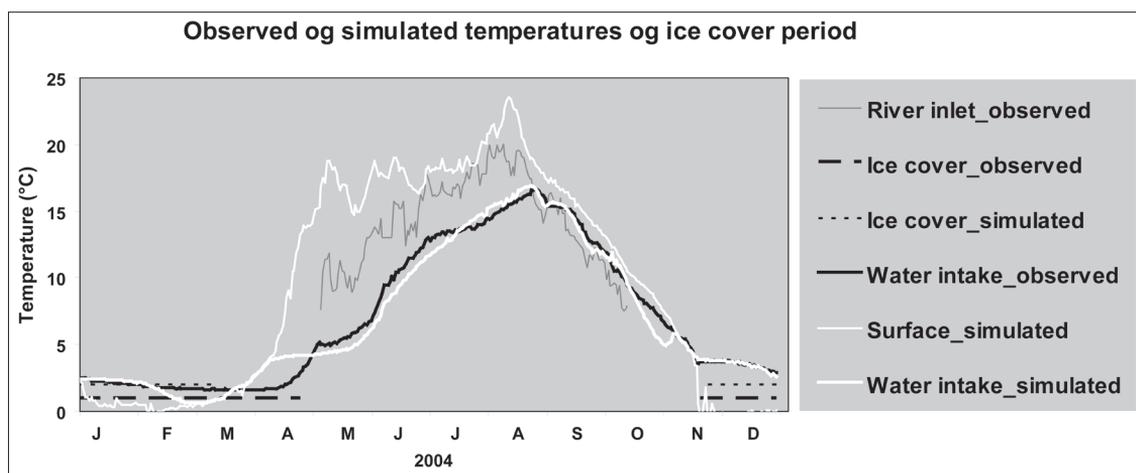
Figure 2. Simulated temperature in the raw water intake was in good approximation to the measured values.
