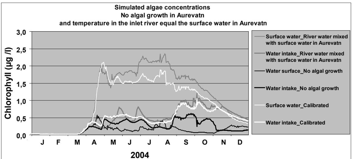
Figure 7. The transport of microalgae with the inflowing river from L. Smaavatn influenced considerably the quality of raw water (explanation, see text). Use of dam overflow (surface discharges) from the upstream reservoirs did not improve the water quality in the water intake.
