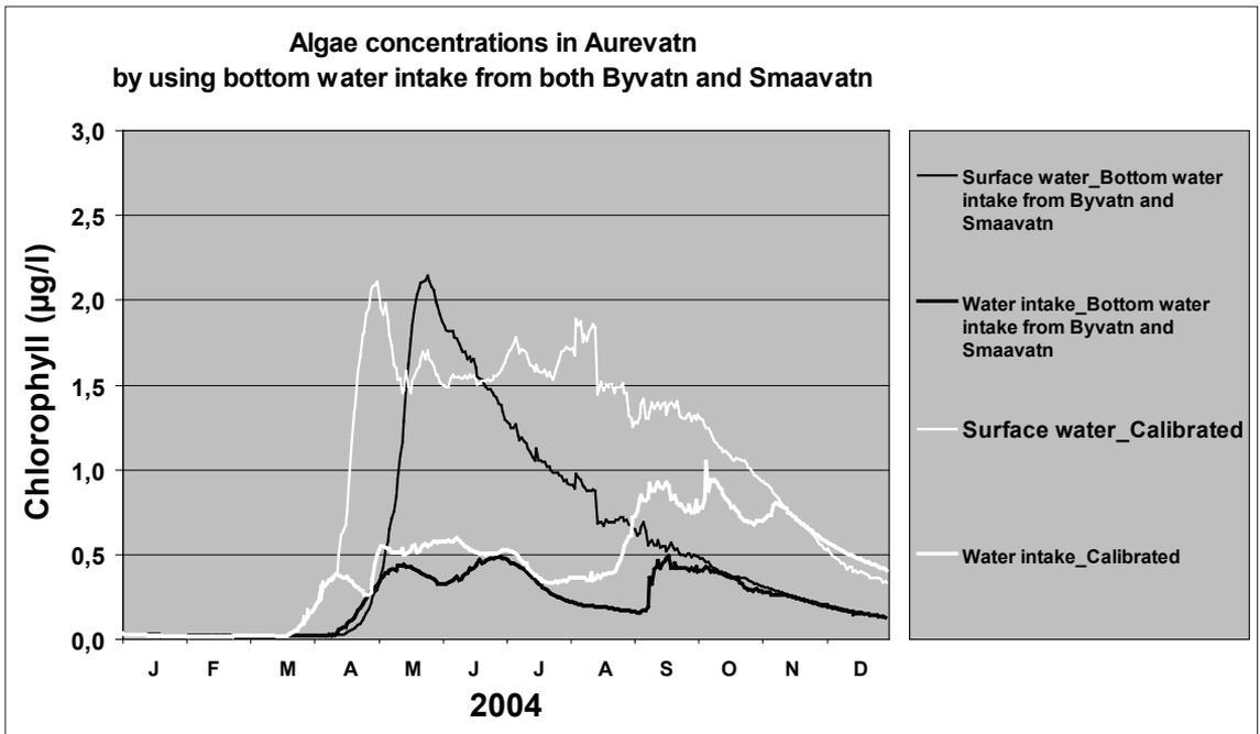
Figure 10. *The hydraulic management of the reservoir system including combined bottom water discharges from L. Byvatn and L. Smaavatn will result in lower concentrations of microalgae in the raw water intake to the water works.*
