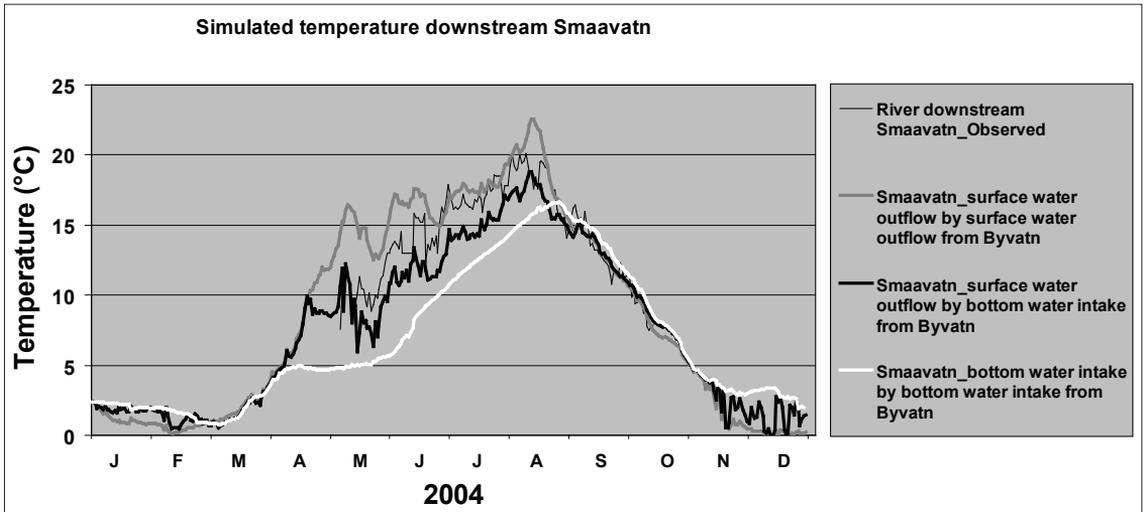
Figure 8. Operating bottom water discharges from the upstream reservoirs (L. Byvatn and L. Smaavatn) will result in low water temperature in the inflowing river to the Aurevatn reservoir.
