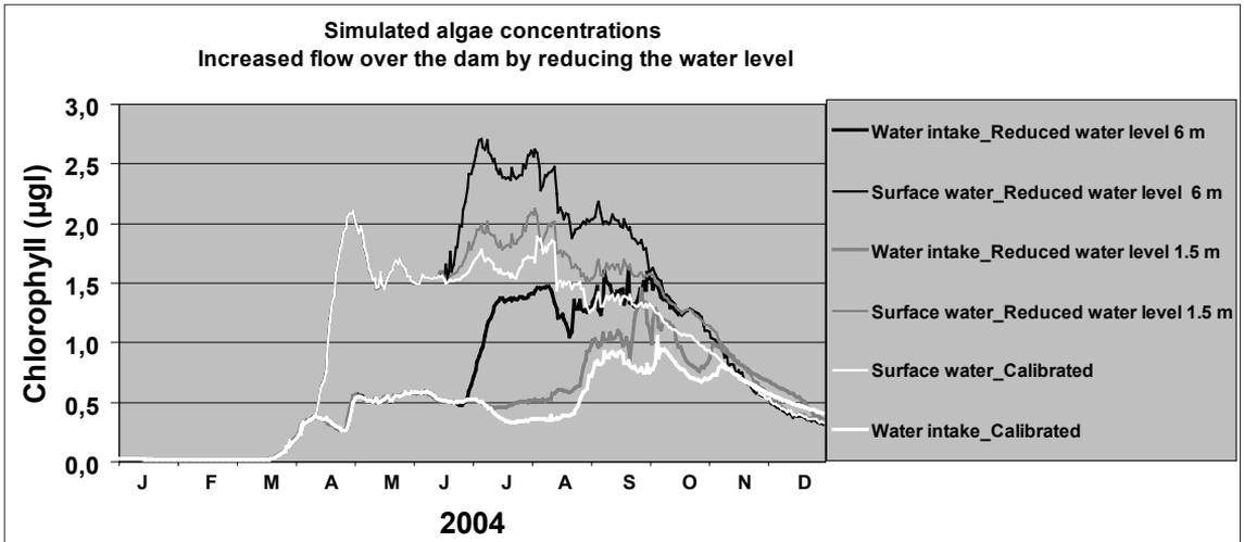
Figure 6. An alternative procedure for a removal of surface water from the Aurevatn reservoir was examined based on reducing the water volume (explanation, see text). The results obtained in the simulation implied increased content of microalgae both in the surface water and in the raw water.
