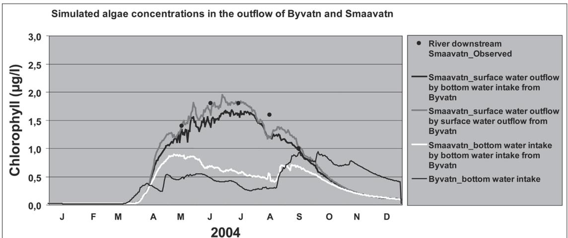
Figure 9. To obtain low concentrations of microalgae in the inflowing river to the Aurevatn reservoir, bottom water discharges from both of the upstream reservoirs (L. Byvatn and L. Smaavatn) should be operated.
