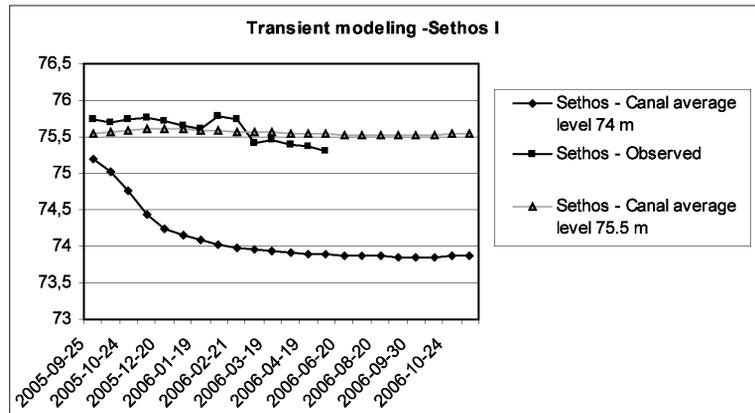
with the same conditions as in the first scenario. The figures 7 and 8 show the results of both temples for observed and calculated groundwater levels.
