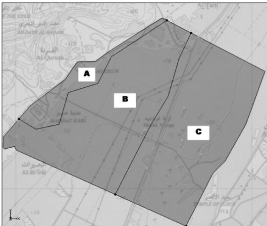
Figure 6. Division of the uppermost Layer 1: Areas A and C mostly consist of silty clay with a low K-value of 1.55 m/day. Area B contains sands and gravels, with a K-value of 35 m/day.
