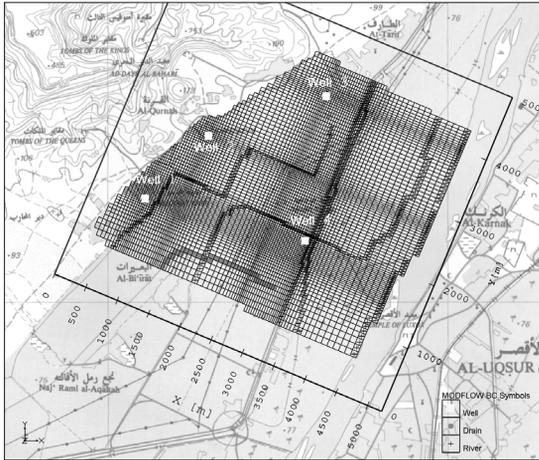
Figure 5. Modelling area with grid showing the location of Wells 1 to 4, the internal canals and drainage, (Graphic aid, GMS 6.0).
