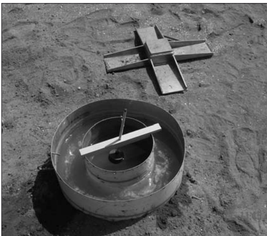
Figure 1. Tools used during the infiltration experiment.
