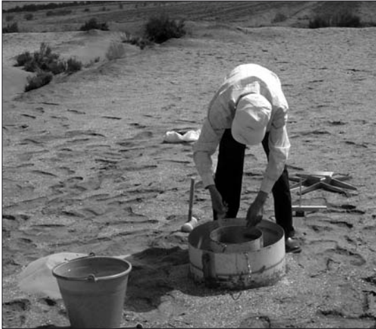
Figure 3. Putting a 2 cm sand layer on the soil surface.
