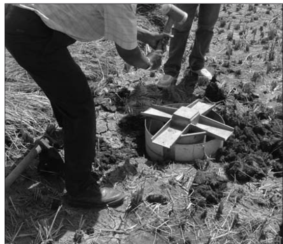
Figure 2. Driving the double ring infiltrometer into the soil.
