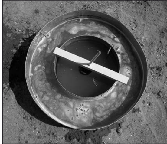
Figure 4. Infiltration rate measurements.
