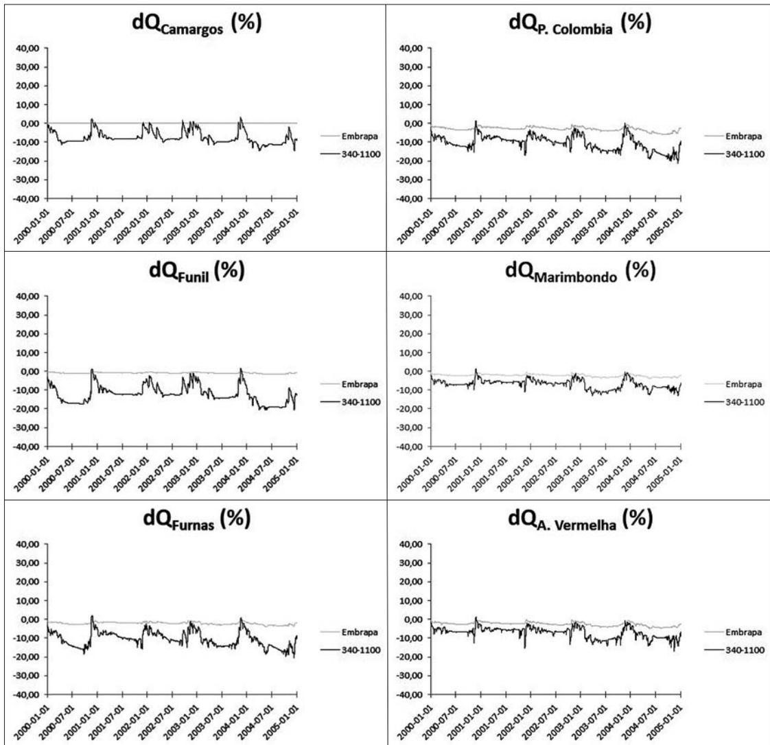
Figure 5. Relative changes in discharge at the HPPs for the 340–1100 and Embrapa scenarios (2000–2004).
