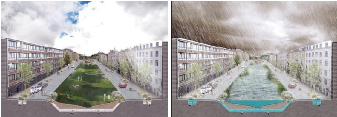
Figure 6. Open storm water handling solution suggested for Sønder Boulevard in Copenhagen (illustration by Copenhagen municipality). Pictures are adopted from Jørgensen (2013) with permission.
