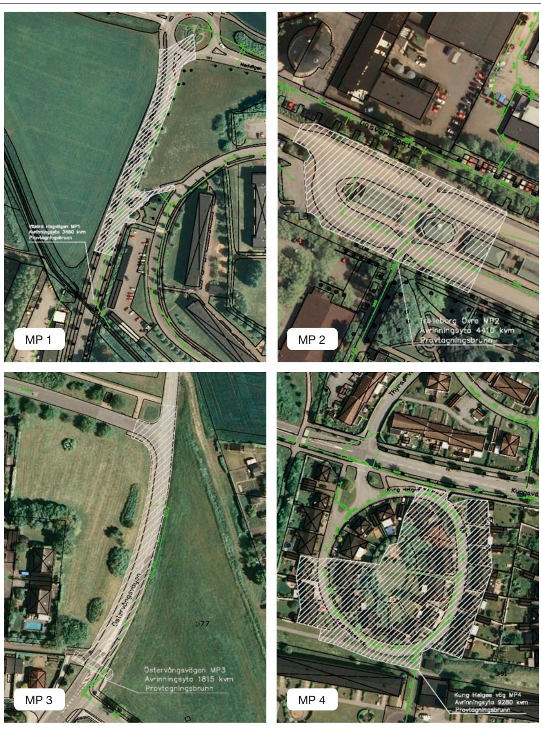
Figure 1. Storm water catchments and sampling points MP1–MP4.
