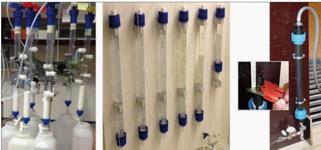
Figure 1. Rapid NOM-fractionation (left) and BDOC columns-in-series set-ups (Eikebrokk, 2014).
