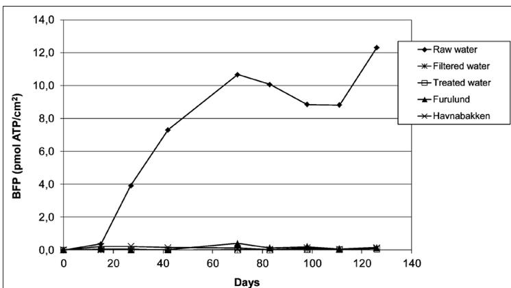
Figure 2. Biofilm formation potential (BFP) during 125 days of biofilm build up in the biofilm monitor.
