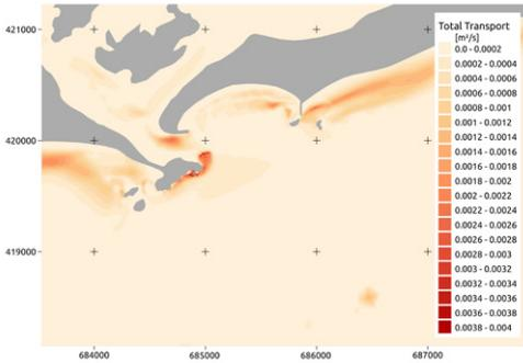
**Figure 8.** Total sediment transport rates at low spring tide and waves from southwestern origin.
