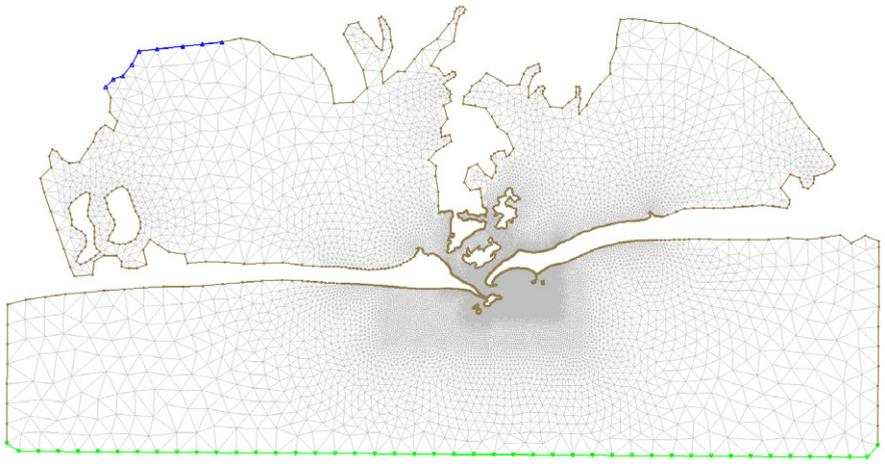
Figure 6. Mesh of the model including set boundaries. Blue represents the river boundary and green the southern boundary.
