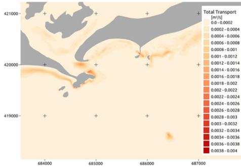
**Figure 9.** Total sediment transport rates at low spring tide and waves with southeastern origin.
