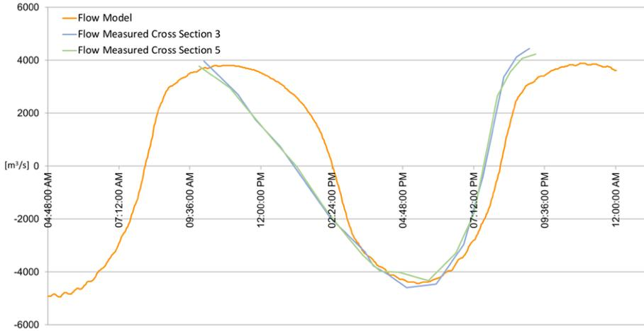
**Figure 7.** Comparison of modeled flow against measurements
