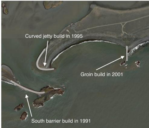
**Figure 2.** Coastal protection structures at the Hornafjörður coastal inlet (NASA Landsat, 2018)
