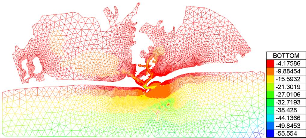
Figure 5. Three dimensional mesh with bathymetry of the modelled area.
