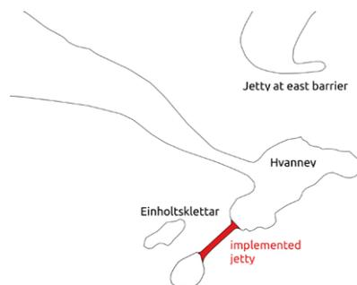
**Figure 10.** Implementation of a jetty to limit sediment transport to the inlet.
