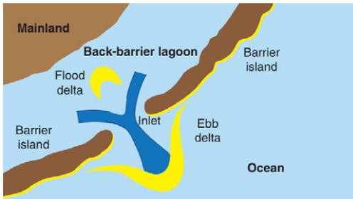
**Figure 3.** Components of a typical coastal inlet (Van de Kreeke and Brouwer, 2017)
