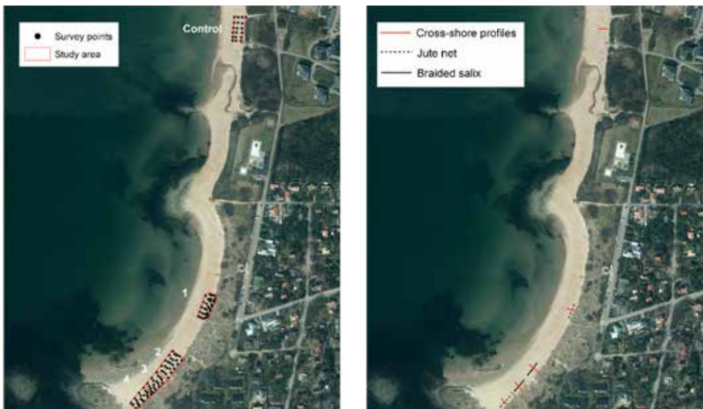
Figure 1: Sand fence sites and survey measurements are shown to the left, while the fences and the cross-shore profiles are seen in the figure on the right. Study areas stretch up to 10 m from the fence in either direction, and profiles vary between 15 and 20 m in length.
