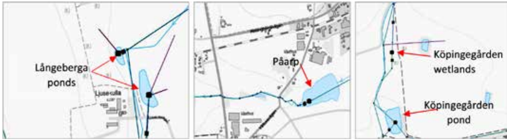
Figure 3. Illustration of the modelled ponds and wetlands in the three different areas, Långeberga, Pårarp and Köpingegården. The darker, straight lines show the model and the lighter lines in the background show location of the watercourse according to the map. The brown cylinders represent ponds and wetlands, while the weirs are represented by a black and yellow square symbol.
