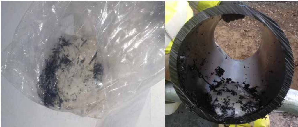
Figure 3. To the left: The white blob (later identified as wheat flour) in incident no 1 was about the size of an orange. The black chips are pieces of the cut PE-pipe. To the right: The blob from incident no 2, later identified as growth of bacteria and fungus around a paper napkin.
