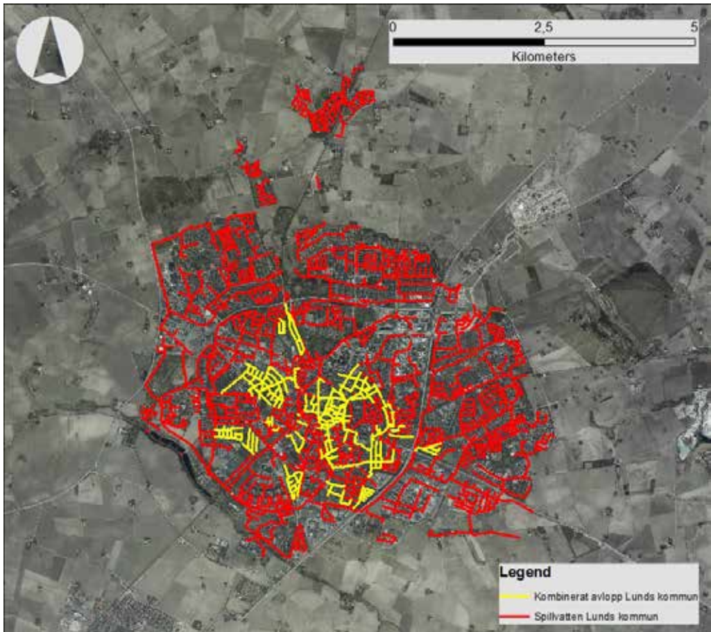
Figure 1. Division of sewer type in Lund. Red indicates separated sewers and yellow indicates combined sewers.
