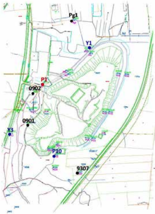
Figure 3. Location of sampling control points at the Bångshagen landfill. Groundwater – points Pg1, 0901, 0902, 9307. Surface water – Y1, Y3, P10. Filtrate - P1.
