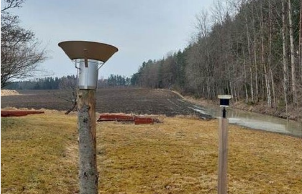
Figure 2. Test of performance of a Netatmo rain gauge, carried out by SMHI. Photo: Mikael Stenström, SMHI.
